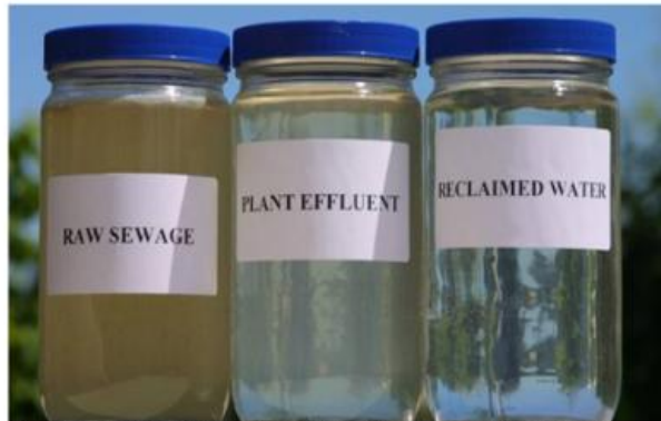
Reclaimed water is not wastewater. The process of reclaiming water uses advanced technologies to filter and remove pathogens and contaminants.
